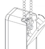
5 Tight chain on the motor , put motor slide groove down, until motor lock on groove, pls choose reasonable chain tension.
